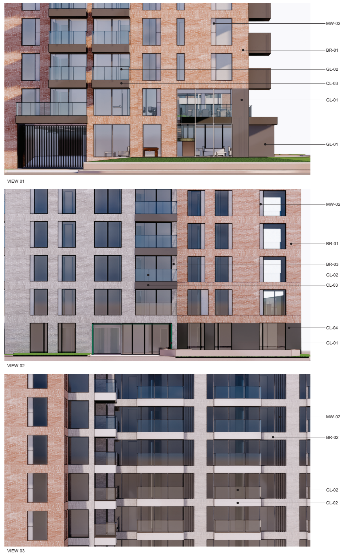
Fig. 35 3D visualisation of proposed Block A with material key and image references
